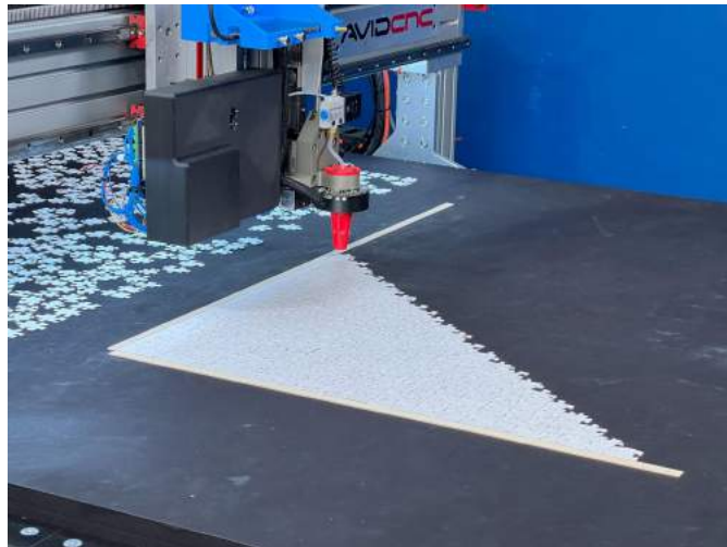
Left: wooden registration strips taped to the table; Right: puzzle robot using the registration strips to place pieces in consistent locations
