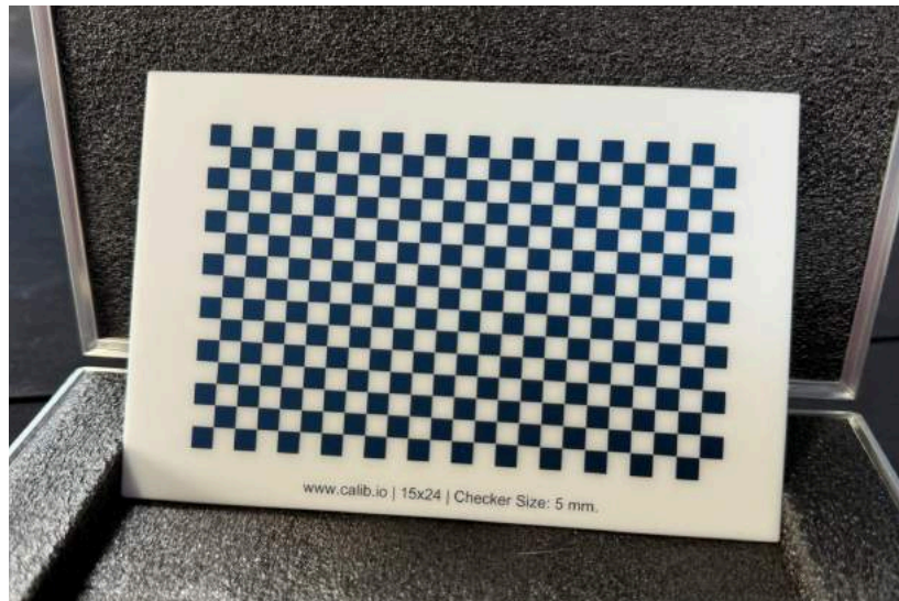
High-accuracy calibration target with 10-micron dimensional accuracy
